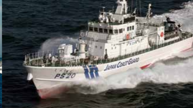
Shinzan, PS-type vessel (180tons) Length overall: 46.0meters Maximum breadth : 7.5meters Gross tonnage : 195tons
