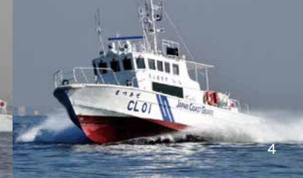
Satsukaze, CL-type craft (20meters) Length overall : 20.0meters Maximum breadth : 4.5meters Gross tonnage : 26tons
