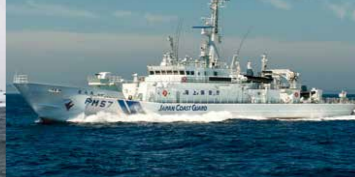
Sorachi, PM-type vessel (500tons) Length overall : 72.0meters Maximum breadth : 10.0meters Gross tonnage : 650tons
