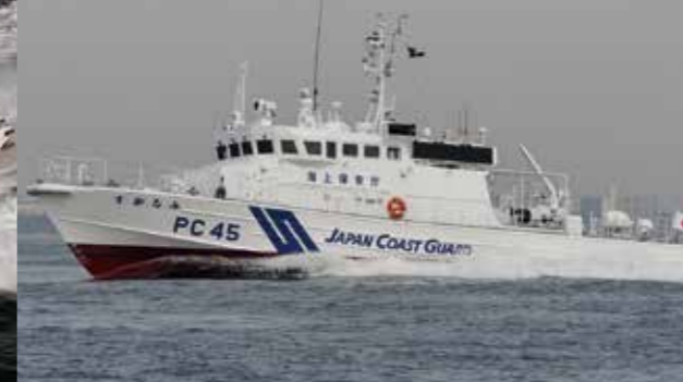
Suganami, PC-type craft (23meters) Length overall: 27.0meters Maximum breadth : 5.6meters Gross tonnage : 64tons
