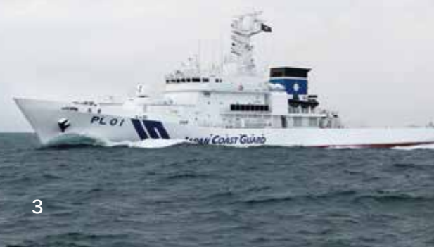
Oki, PL-type vessel (1,000tons) Length overall : 96.0meters Maximum breadth : 11.5meters Gross tonnage : 1,500tons
