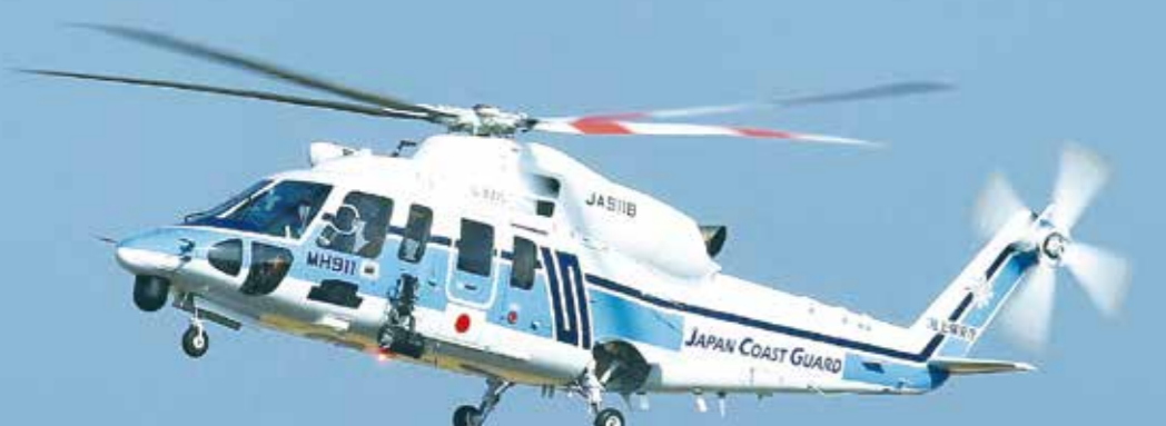
Sikorsky76D helicopter Length overall : 15.97meters Height : 4.41meters
