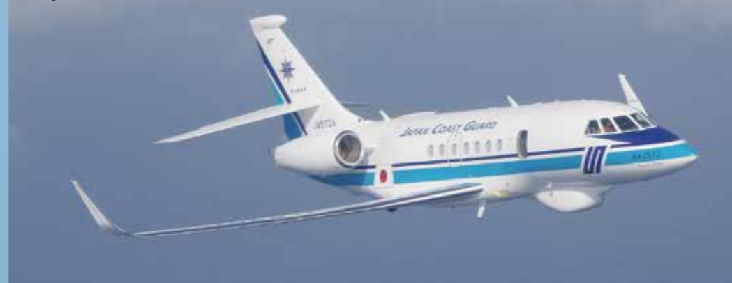
MAJ Falcon2000 Length overall : 20.23meters Full width : 21.38meters Height : 7.18meters
