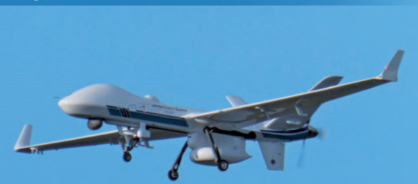
Sea Guardian Length overall : 11.70 meters Full width : 24.00 meters Height : 3.70 meters
