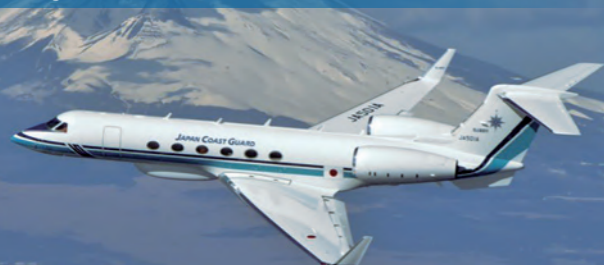
Gulfstream V Length overall : 29.39 meters Full width : 28.49 meters Height : 7.89 meters
