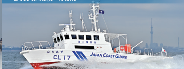
Nachikaze, CL-type craft (20meters) Length overall : 18.0 meters Maximum breadth : 4.3 meters Gross tonnage : 19tons
