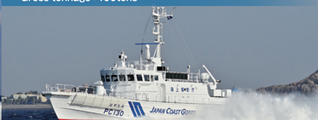
Hayanami, PC-type craft (30meters) Length overall : 32.0 meters Maximum breadth : 6.5 meters Gross tonnage : 100tons
