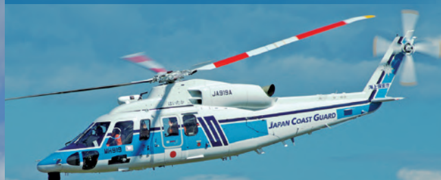
Sikorsky 76D Length overall : 15.97 meters Height : 4.41 meters
